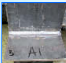
Photo 3 Shows a single pass dry fillet weld
